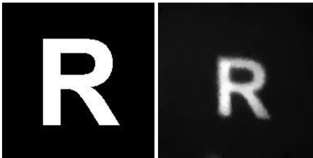
Figure: 16384 ( n ) pixel image, reconstruction with 1600 ( m ) measurements (Wakin et al., 2006)
