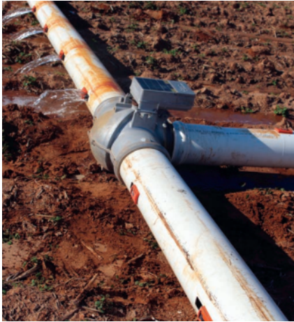
Figure 2.4a: Automatic surge valve, connected to a water supply inlet and outlet pipes [12].
